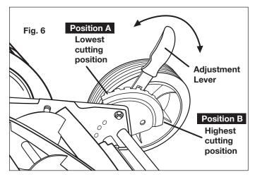
**4.** Other cutting heights are achieved by moving the adjustment levers to the settings between the highest and lowest positions.
