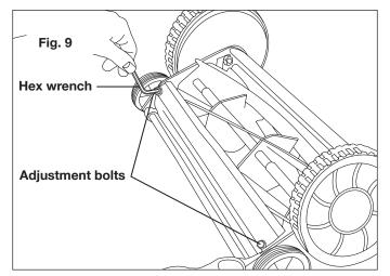
⚠ WARNING! Do not overtighten the adjustment screws as this could damage the cutting bar. Both screws must be tight on final adjustment.
