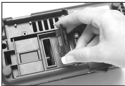
Figure 18. Removing cover under base to clean out metal dust (See Normal Maintenance section).
