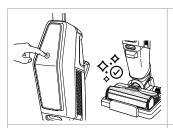
4. Push the Clean Out Cycle Button to start the 40-second cycle.
