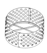
Step: 3 Attach Top Ring (Item 5) to opposite side of step 2 using screws (Item A) loosely. All Side Meshes should sit inside the Top Ring. Make sure all connectors are in position before tighten all screws from Step 2 and
