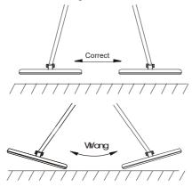
(2) Sweep your search coil as following picture, move the search coil right and left in an arc line. For not missing any target, it is better to keep the distance from search coil to the ground about 1-2 inches (closer to the earth for smaller target) and the distance between two neighboring arcs is about 15-20cm. Please move slowly and it should be parallel between the arc lines in case the object can be missing.
