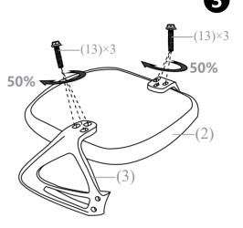
Note 1: The "Front" mark on the Armrests and the "Front" mark on the Seat Cushion should be in the same direction.
