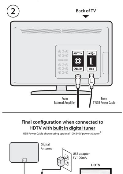
**C.** The amplifier requires power to operate properly. Plug the round end of the amplifier's 5ft long USB power cable into the amplifier (as shown in figure **1**). Then insert the USB plug into an open USB port on the back of your TV (see figure **2**). If no USB port is available, use the supplied power adapter to power the amplifier through any standard 110V outlet (see this option in figure **3**).
