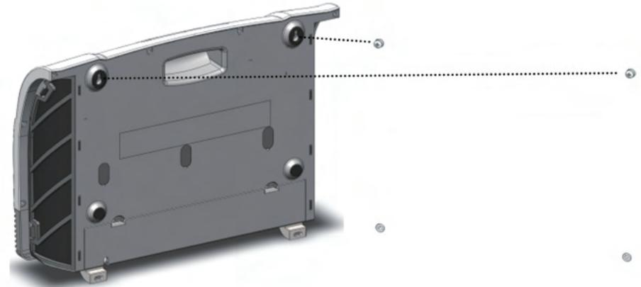
4. Screw in final 2 screws into base anchor holes to secure heater onto wall
