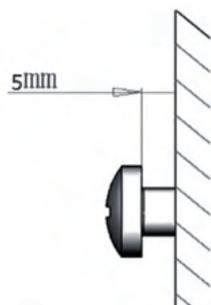
2. Drill holes for included anchors and screws. Insert top 2 screws first
