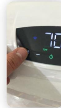
While the heater is plugged in and turned on, press and hold the wifi/sun symbol on control screen for 5 seconds. You should hear a beep and see a wifi symbol start blinking in a blue color
