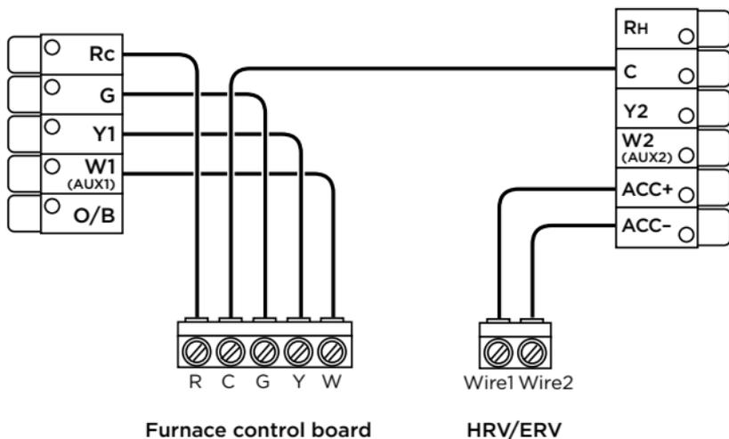
**Note:** To determine which wires from your ERV/HRV need to be connected to the ACC+/ACC- terminals on your ecobee3, you will need to refer to your ERV/HRV manual. The two wires will be listed under configurations that enable “optional auxiliary control for high speed fan” or “dry contact timer configuration”.
