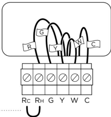
Discard any jumper wires between Rh, Rc, or R. Your ecobee3 does not need them.
