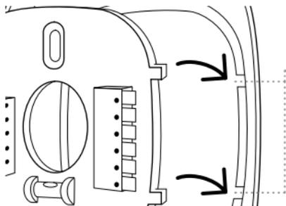
Insert the back plate using the tabs on the right as a guide. It will snap into place when correctly inserted.
