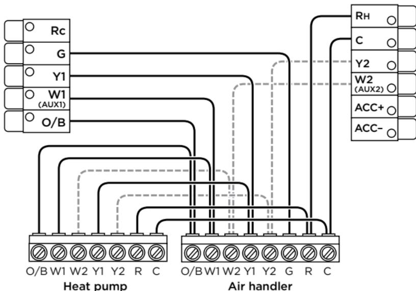
**Note:** Do not jumper R<sub>c</sub> or R<sub>h</sub>, ecobee3 does this automatically. R can go into either R<sub>c</sub> or R<sub>h</sub> terminals on your ecobee3.
