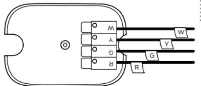
4. Open up the PEK. It has two rows of terminals (one side is for thermostat connections, the other side, pre-wired, is for the control board connections).
