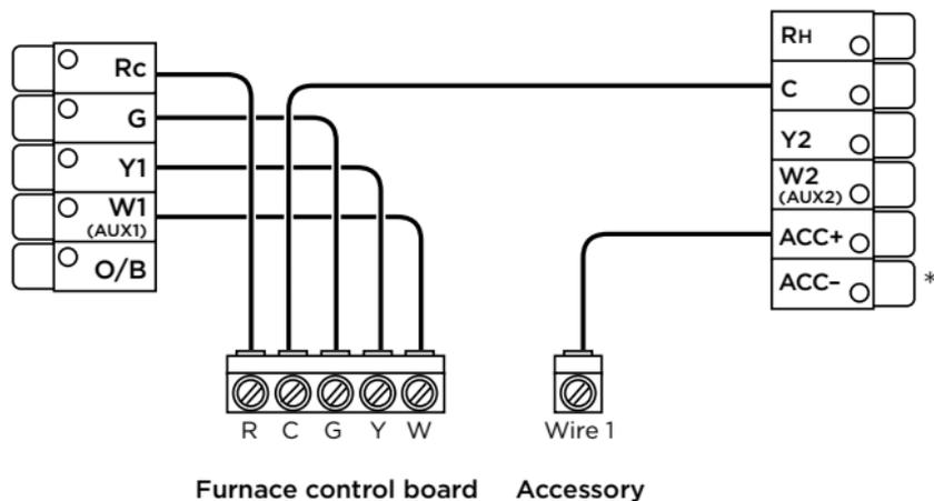
\*ecobee3 automatically connects Rc to ACC- when 1-wire configuration is selected during accessory setup.
