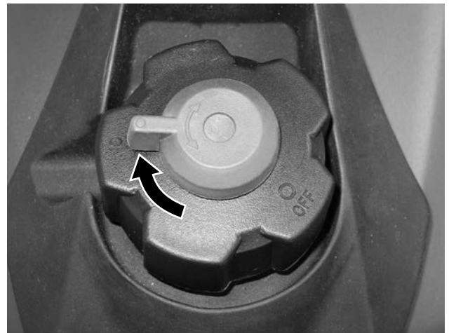
Figure 27 – Fuel Tank Vent
