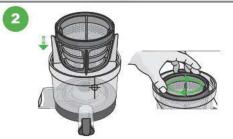
Place the assembled silicone brush and screen into the juice bowl. Move it left to right until it clicks into place.
