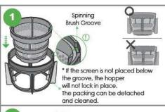
Assemble the screen. The top of the screen must sit below the grooves on the spinning brush, as shown in the picture. Otherwise, the chamber set will not close properly.
