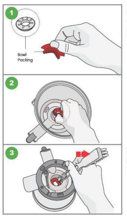
As shown to the left in the dotted circle, let the protrusion part on the bowl packing face upward and hold it, like pinching, with your thumb and index finger.
