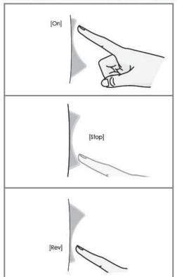
To STOP the operation, press the [Rev] button quickly. The auger will rotate slowly then stop. After the auger rotation stops completely, you can press [ON] to continue operation as normal or hold down the [Rev] button to push ingredients upward.
