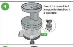
Place the hopper onto the juice bowl. Turn the hopper clockwise until it is locked completely.
