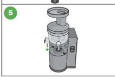
Mount the assembled juice bowl chamber onto the motor base.
