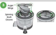
Next place the auger inside the screen. Align the augers wings with the grooves on the spinning brush.
