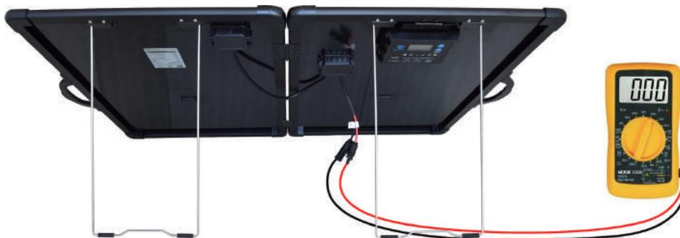
Set your multi-meter to measure DC voltage and put the red probe on the red positive MC4 cable (7a, Table 1) and the black probe on the black MC4 cable (7b, Table 1) and make sure the connections are secure. The open-circuit voltage should be displayed on your multi-meter and it should be around 17.6V-23V. This is your solar panel's voltage without going through the charge controller.
