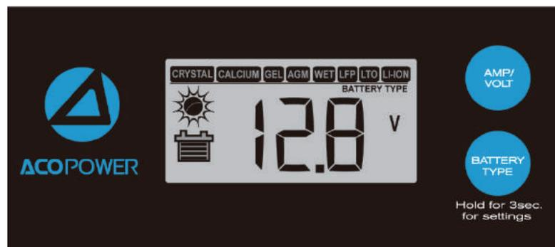
Press **BATTERY TYPE button** and hold for 3 seconds to go into your battery type selection mode, the battery type you select will be shown on the LCD meter, the default setting is AGM Battery; the controller will automatically memorize your battery type setting.
