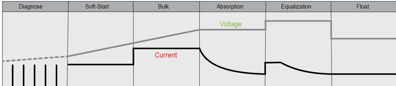
**Diagnose \*** – Only for Lithium battery type, subjected to the Lithium battery initial voltage then determine going to Soft start or Bulk charge; if the Lithium battery is protected by BMS, the controller will automatically send the signal periodically to the battery terminal to activate the BMS against protection.
