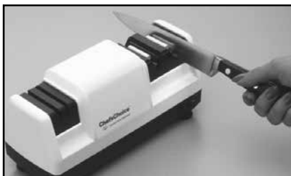
Stage 3— Six (6) passes through each slot (left and right HONING slot). Alternate each pass.
