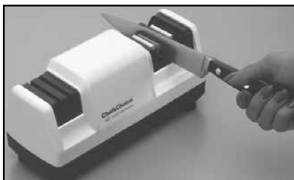
Stage 2— Six (6) passes through each slot (left and right SHARPENING slot). Alternate each pass.
