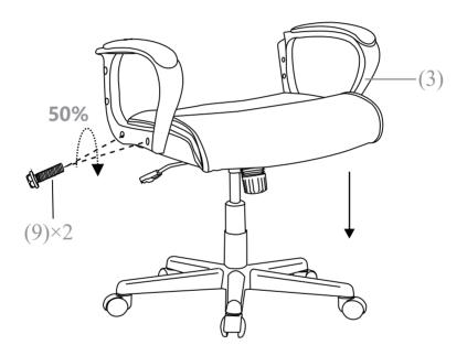
Note 1: The "Front" mark on the Armrests and the "Front" mark on the Seat Cushion should be in the same direction.
