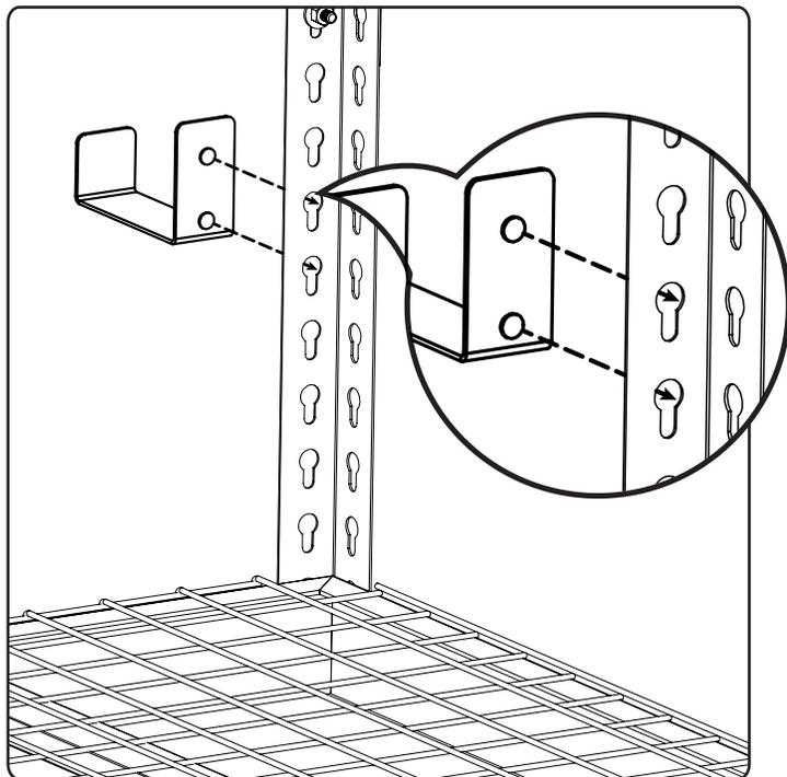
**2** Slide the J-Hook down to align the rivet nubs with the bottom of the keyhole slots.
