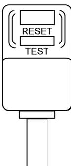
Your portable air conditioner is supplied with a Leakage-Current Detection and Interruption (LCDI) plug. This plug reduces the risk of fire due to arcing faults in the power supply cord. Please follow the instructions below to ensure that LCDI plug works properly.
