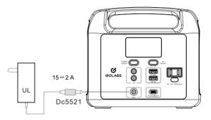
Plug the original adapter into the machine's DC input port and you will see the battery indicators on the screen blink.
