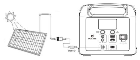
A.Place your solar panel where it will get as much strong direct sunlight as possible. B.Connect the output port of the solar panel with the input port of the product to start charging. You will know the product is being charged when the LCD display indicators blink. The product is fully charged when all battery indicators stop blinking and remain solid
