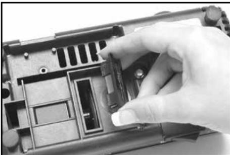
**Figure 16.** Removing cover under base to clean out metal dust. (See Normal Maintenance section)
