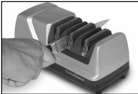
Figure 6. Honing in Stage 2 (left slot).
