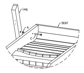
6) Turn chair over. Attach Leg to Seat using bolt C and washer A. 7) Repeat on other side.
