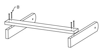
3) Attach Back Support Rail to Back Support Sides with four B screws
