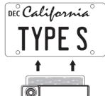
Peel off the cover of the double-sided tape from the International Mounting Plate, and attach the license plate to the Wireless Backup Camera
