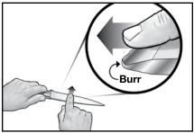
Figure 5. Develop a distinct burr along knife edge before stropping in stage 2. Burr can be detected by sliding finger across and away from the edge.
