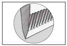
Figure 8. Retention of larger microflutes adjacent to edge helps when cutting fiberous foods.
