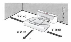
Plug in the power cord and push the charge base against the wall. Place the rounded side of your Neato against the metal contacts on the charge base. 4
